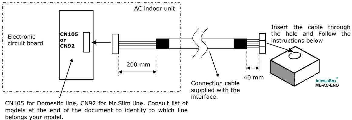
**Figure 2.1** Device connection diagram
