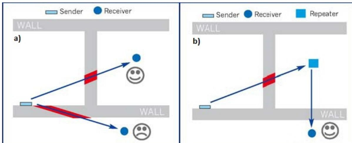
**Figure 2.4** Penetration angle
