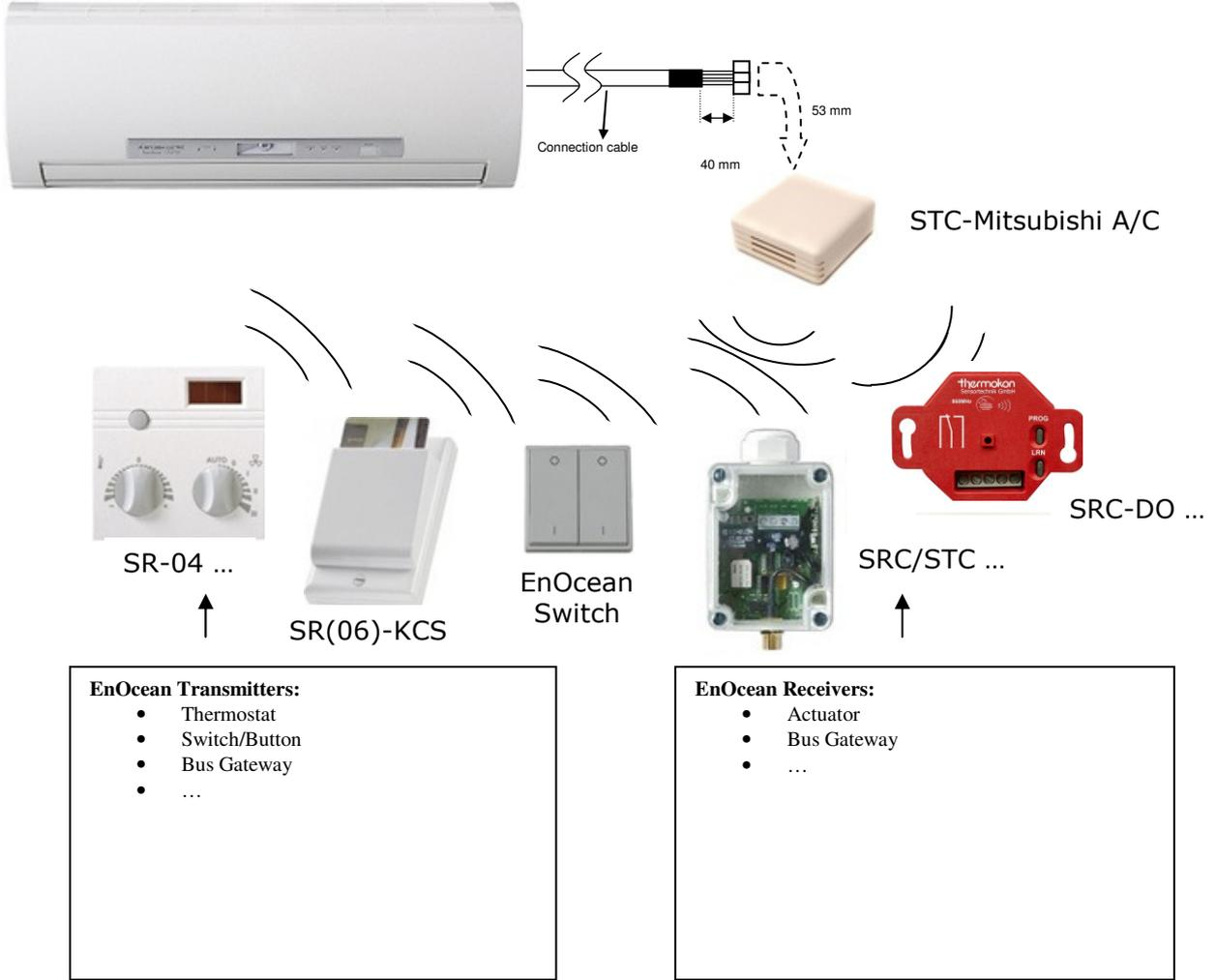
**Figure 1.2** Example of STC-MITSUBISHI A/C control or actuation devices
